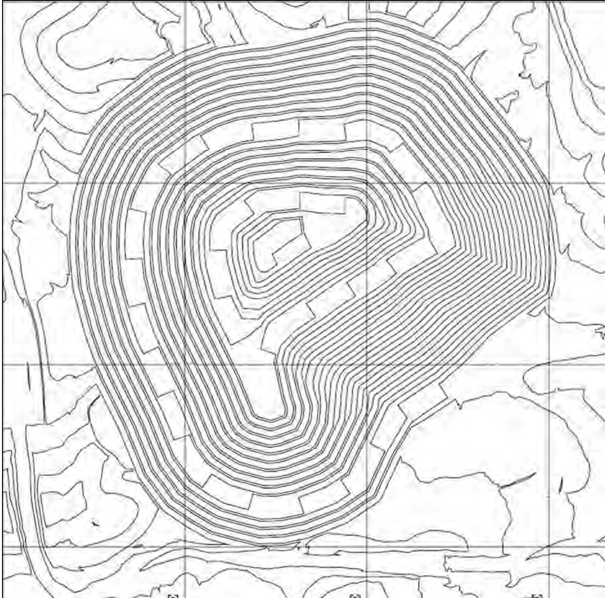
Figure 15-2: Final Pit Design for Mine Plan and Mineral Reserve
