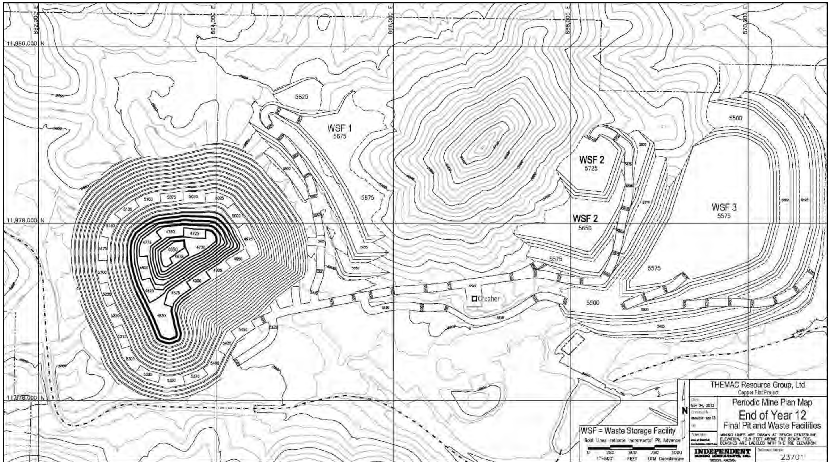
Figure 16-13: Periodic Mine Plan Map – End of Year 12
