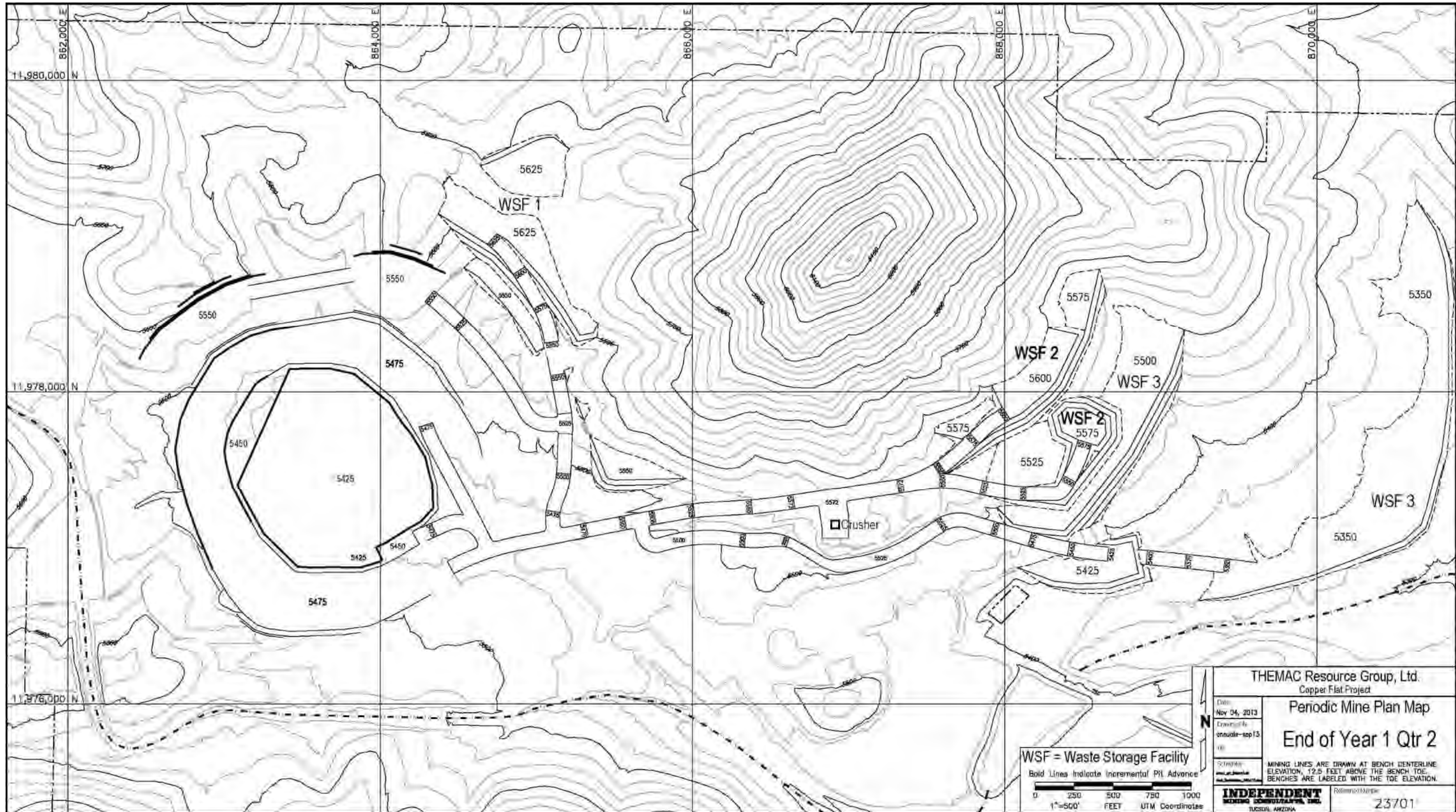
Figure 16-4: Periodic Mine Plan Map – End of Year 1 Q2
